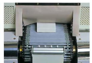
Covering for rollers in shrink tunnels
